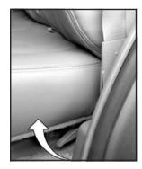
2. Pull the seatback release lever upward and pull the seatback up and fold it down until it is flat. Escalade lever shown, Escalade ESV lever similar. On the Escalade ESV models, first remove the headrest and store it on the top of the seat cushion as shown next.
